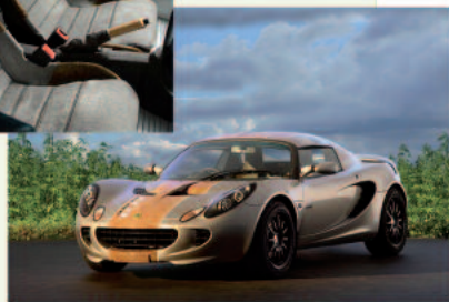
Sports car Lotus Eco Elise, in the main made from different natural fibre compounds, hand lay-up, vacuum bagging and RTM (UK). Pictures: Lotus Cars
