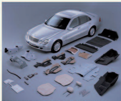
50 Natural fibre parts for Mercedes E-Class (Germany). Picture: Daimler AG
