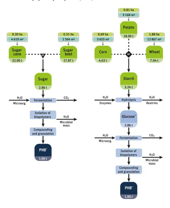
\* Conversion rates: Starch – Glucose 90 % fermt. Sugar – PHB 35 %
