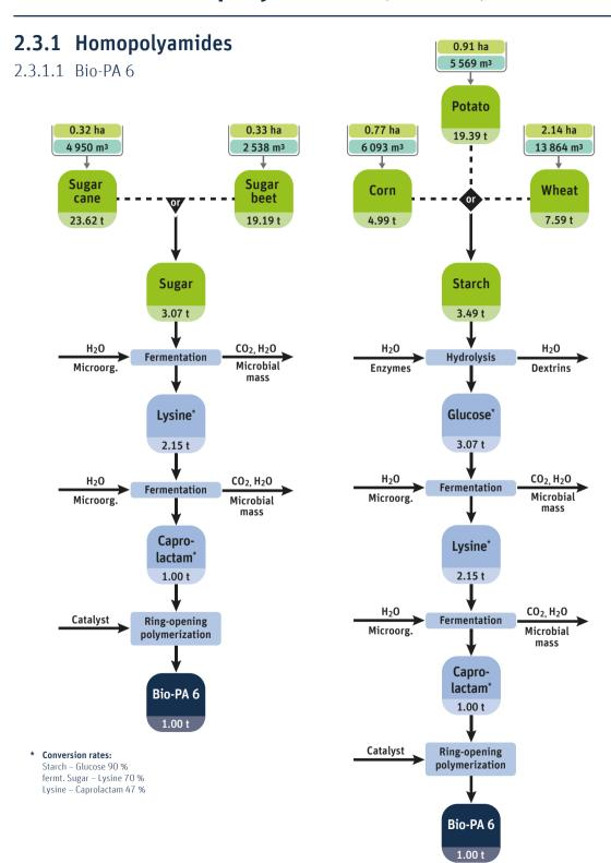
**Bio-PA 6 – Feedstock requirements in t** (different feedstocks)
