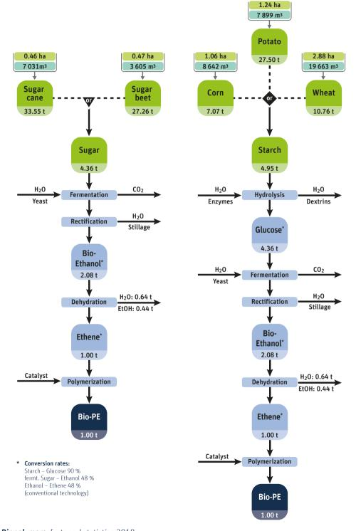
**Bio-PE – Feedstock requirements in t** (different feedstocks)
