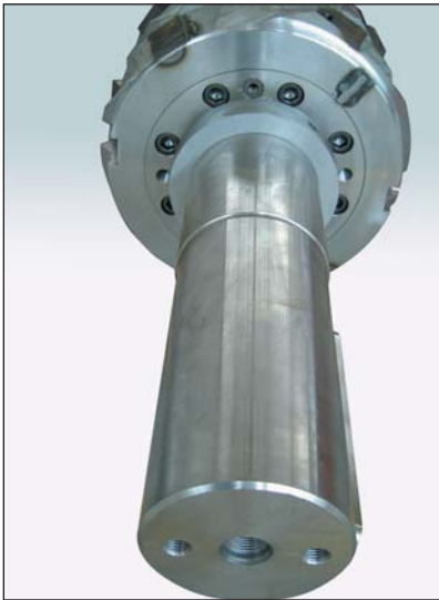
Photo 2: Single-Shaft Shredder, Series WLK – Screw-Type Shaft Journal
