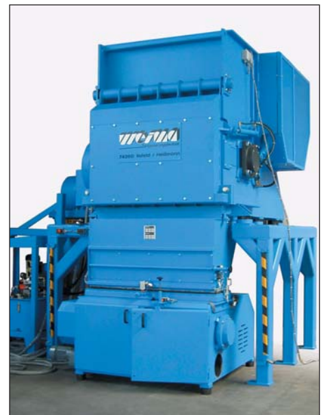
Photo 1: Two-Stage Size Reduction with Universal WLK Shredder and NZ Reshredder, arranged above each other
