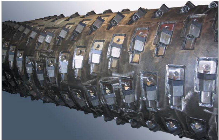
Photo 3: Single-Shaft Shredder, Series WLK – Rotor with Hardox Plating (In-house photos: WEIMA Maschinenbau GmbH, Ilsfeld)
