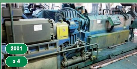
Lot 33 : extrudeuse bi-vis twin screw extruder COMAC 60/42D
