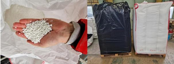
Water absorption and moisture uptake are very low (0.2%). Water sorption occurs only on the surface of the material, allowing use in environments with variable relative humidity without dimensional changes or alterations in mechanical properties. During processing, difficulties may arise due to moisture condensed when transferring material from a colder to a warmer environment.
